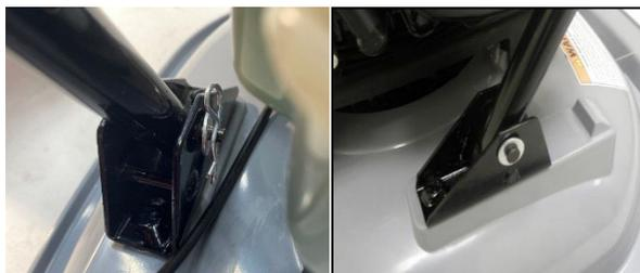
3. Attach the **upper handle** section to the lower handle section – with the stop lever facing forward – using the bolts and knobs as shown:
