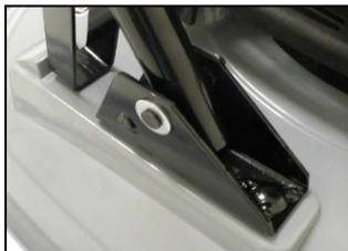
2. Secure the handle by inserting the pins on each side and securing with the spring cotter pin. Note: The spring cotter pin will be on the inside, closest to the engine.
