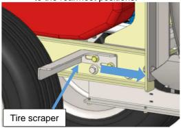
[3] Pull out the axle completely. Switch the axle at the top and bottom position, and insert in the axle until the original tread is achieved.
