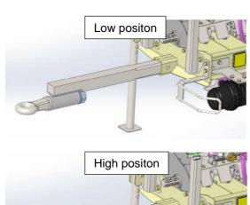
[3] Keep the hitch length as short as possible to the extent that it does not contact the tractor. You can adjust the length of the hitch by removing the two bolts securing the hitch. After the adjustment, securely tighten the bolts (torque: 117 N•m).
