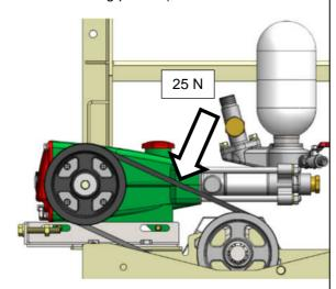
When adjust the belt tension remove belt cover. The cover is secured with two bolts.
