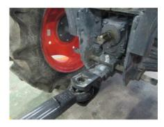
[4] Carefully move the tractor forward to separate the draw bar from the hitch.
