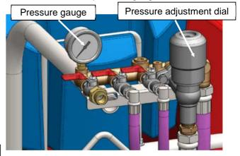
To stop spraying or end the spraying session, turn the pressure adjustment dial counterclockwise until it stops, to lower the pressure, and then turn off the PTO.
