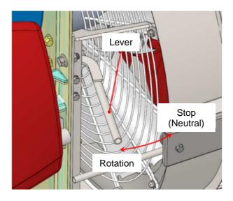
If it is difficult to switch the lever to the rotational position of the fan, turn the universal joint little.
