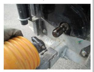
[2] Install the stand on the machine. Install the stand at positions where the hitch does not contact the draw bar. Choose the position of holes where the hitch does not contact the draw bar.
