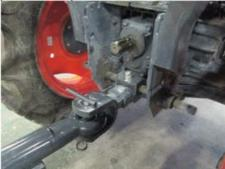
[5] Confirm that the machine is securely connected to the tractor, and then remove the stand.
