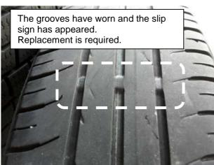
Caution ● If the tire pressure is too high, the tire tends to wear unevenly. If the tire pressure is too low, a flat tire occurs easily.
