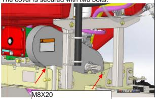
Tightening torque: 20 N·m
