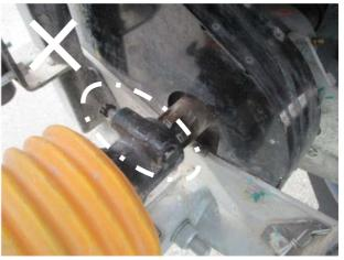
[3] When the shafts have been connected, be sure to secure the joint cover with a chain to prevent it from turning.
