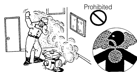
Be careful of ventilation and combustibles!
