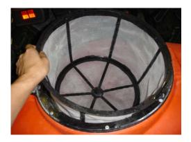
The strainer of chemical tank will filter rubbish when you feed water or mixed chemical.
