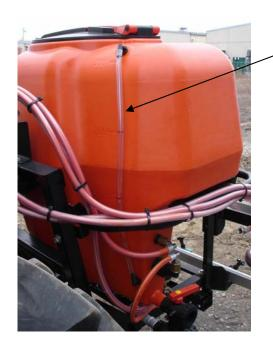
Measurement tube for remain chemical
