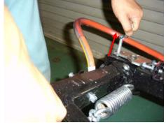
(3)Remove side boom from boom holder, open the boom for 20degree, and insert shaft lock pin where upper & lower pin hole are coincident.
