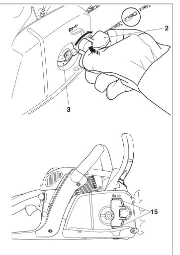
Release the sprocket guard chain tensioner until it turns freely, then fold it in between protective ribs (15) as shown in the illustration.
