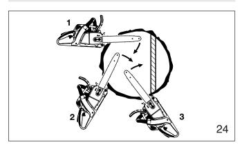
For the sectioning method (fig. 24) make the first cut with the guide bar fanning in toward the hinge. Then, using the bumper spike as a pivot, reposition the saw for the next cut. Avoid repositioning the saw more than necessary. When repositioning for the next cut, keep the guide bar fully engaged in the kerf to keep the felling cut straight. If the saw begins to pinch, insert a wedge to open the cut. On the last cut, do not cut the hinge.
