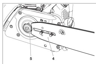
Put the guide bar (4) on and push it against the sprocket (5).
