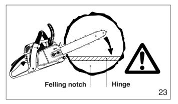
Then, determine the placement of the felling notch (fig. 21). The felling notch when properly placed determines the direction in which the tree will fall. It is made perpendicular to the line of fall and should be as close to the ground as possible. Cut the felling notch to a depth of about one-fifth to one-fourth of the trunk diameter (fig. 22). It should be in no case higher than it is deep. Make the felling notch very carefully.
