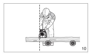
Position the chain saw in such a way that your body is clear of the cutting attachment whenever the engine is running (fig. 10).
