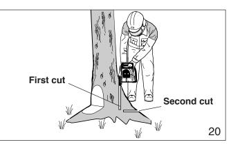
If the tree has large buttress roots, cut into the largest buttresses vertically first (horizontally next) and remove (fig. 20).
