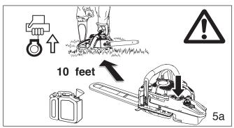
Wipe off any spilled fuel before starting your saw and check for leakage.
