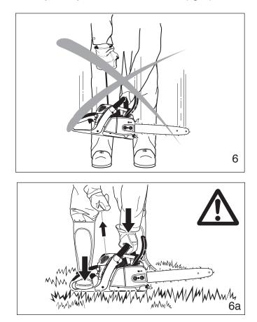
Place the chain saw on firm ground or other solid surface in an open area. Maintain a good balance and secure footing. Place your right foot through the rear handle opening and firmly grasp the front handle with your left hand (fig. 6a).
