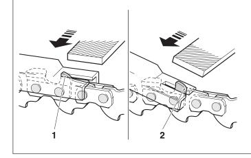
After having sharpened the chain, the height of the depth limiter must be checked by means of a chain gauge. See "Accessories" for the order number.
