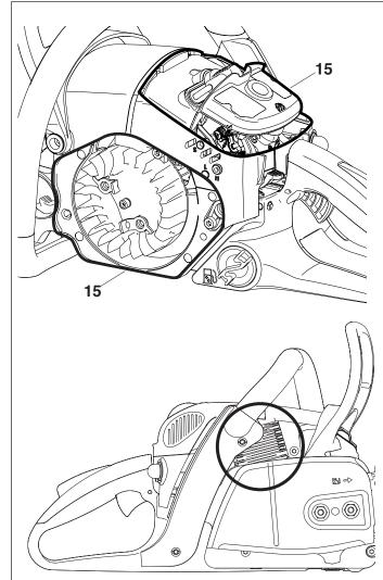
Cleaning the air filter compartment / fan compartment
