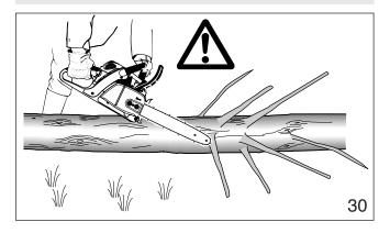
Start limbing by leaving the lower limbs to support the log off the ground (fig. 30). Always cut from the top of the limb. Do not underbuck freely hanging limbs. A pinch may result or the limb may fall, causing loss of control. If a pinch occurs, stop the engine and remove the saw, by lifting the limb.
