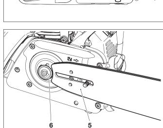
Put the guide bar (5) on and push it against the sprocket (6).
