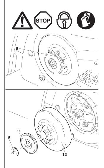
Check the sprocket before mounting a new chain.
