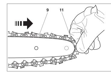
Pull the chain (9) around the sprocket nose (11) of the guide bar in the direction of the arrow.
