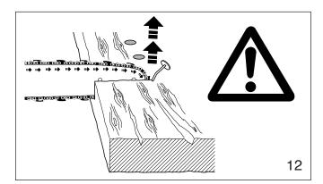
This reaction can occur in a fraction of a second and under some circumstances, cause the guide bar and chain to strike the operator with enough force to cause severe or fatal injury. It may also occur during limbing. It also occurs when the nose of the guide bar is pinched unexpectedly, unintentionally contacts solid material in the wood (fig.12) or is incorrectly used to begin a plunge or boring cut.
