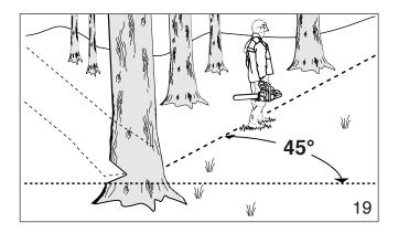
Then, establish a path of escape and remove all obstacles. This path should be opposite to the planned direction of the fall of the tree and at a 45° angle (fig. 19). An alternate path must also be selected. Place all tools and equipment a safe distance away from the tree, but not on the escape path.
