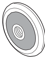
Water intake strainer
